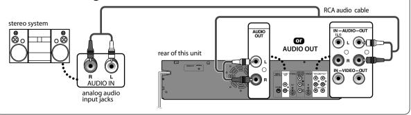
Supplied cables used in this connection are as follows: RCA audio cable (L/R) x 1
