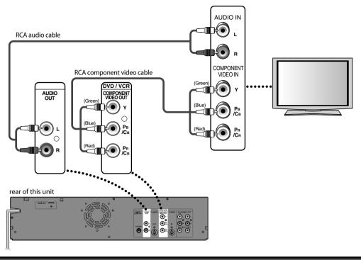
Supplied cables used in this connection are as follows: • RCA audio cable (L/R) x 1 Please purchase the rest of the necessary cables at your local store.
