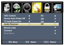
Press down ▼ arrow button to highlight Audio Receiver. Press the ▼ arrow button to select On -Off.
