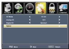
• Press down ▼ arrow button to highlight **Option**. Press the ▶ arrow button to enter a menu with options to customize text fonts, colors and opacities.
