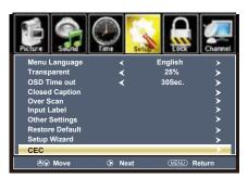
Press the down ▼ arrow button to highlight CEC then press the ► arrow button to highlight CEC Control.
