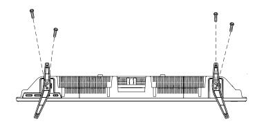
Insert 4 screws (provided) through the holes in the bottom of the base into the post holes and tighten securely. Do not over-tighten.
