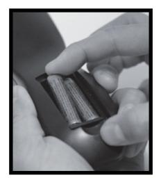
• Place two (2) "AAA" batteries into the battery compartment with the "+" and "-" ends facing as indicated.
