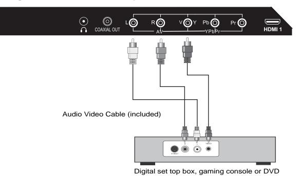
**NOTE:** The yellow A/V cable plugs into the green input labeled Y/V on the back of the TV
