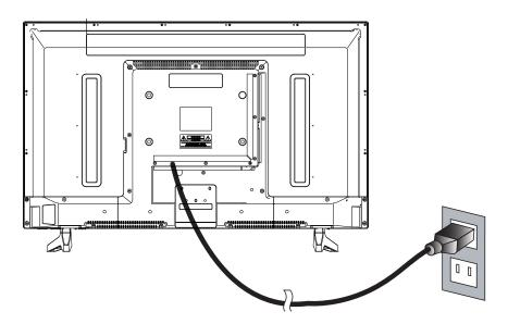
• Connect the power cord to a properly grounded AC outlet.
